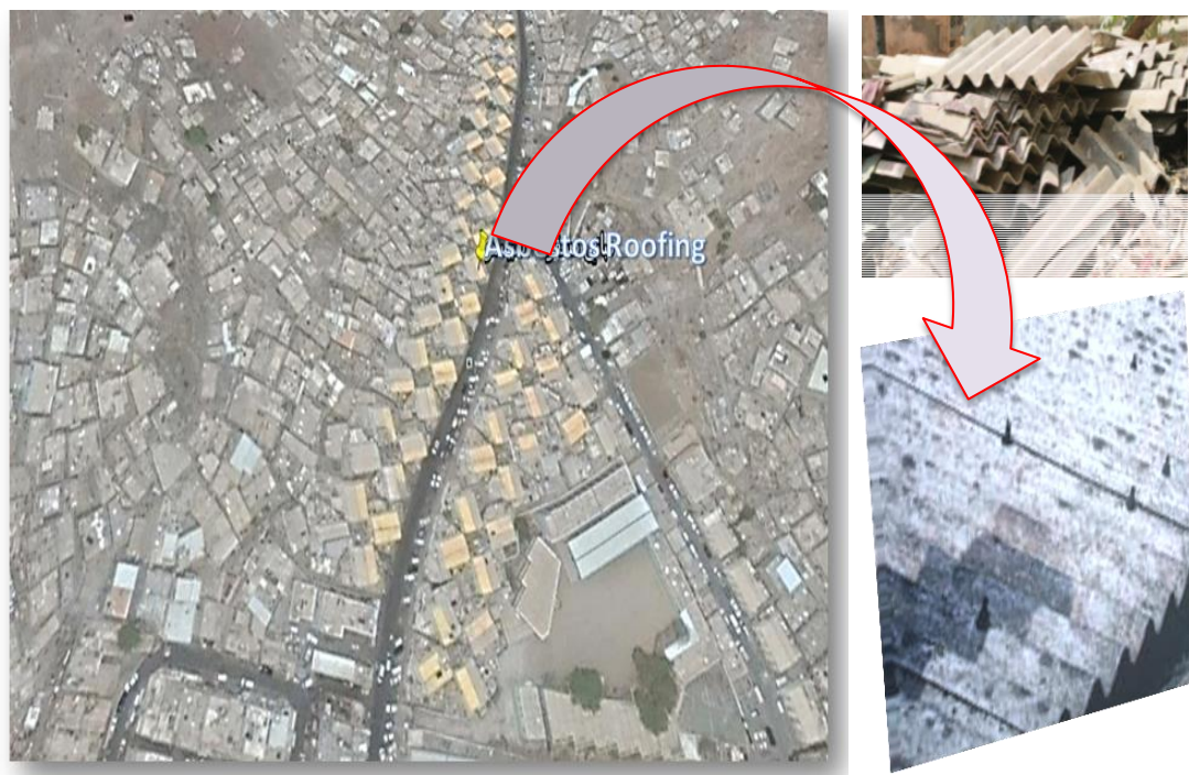
Figure (2) Houses (yellow color) covering asbestos cement corrugated roofing, in Al-Qalluah Town- Aden
