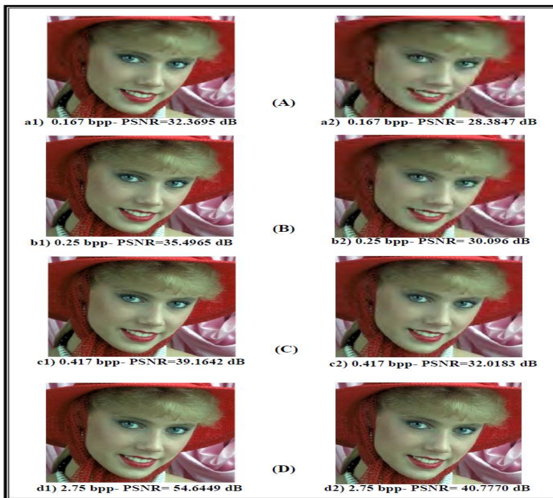
Fig 12 HELEN image with wavelet image compression (a1,b1,c1,d1) & JPEG 2000 (a2, b2, c2, d2)
