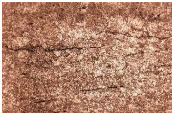
Figure (10) Microstructure of the joint made of S420G2+M steel by local dry chamber method and arc welding with solid wire electrode; numerous cracks in the joint HAZ. Mag. 200 × (Fydrych, Rogalski, & Łabanowski, 2014)
