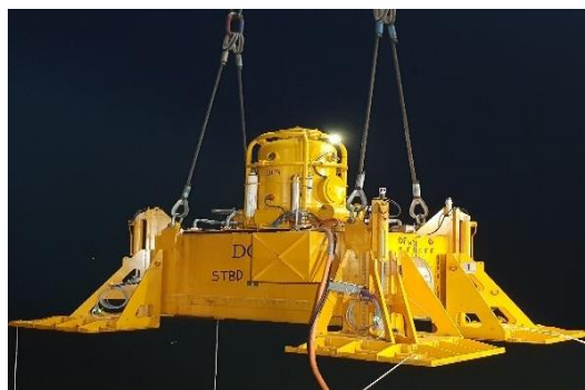
Figure (4) welding habitat used for performing dry underwater welding (Diving, 2021)
