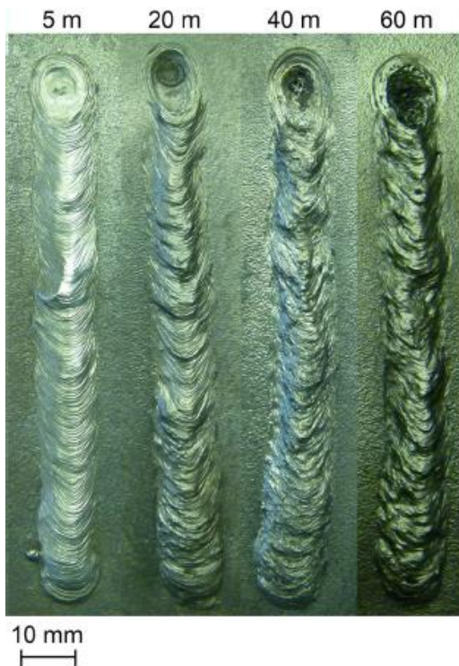
Figure (14) influence of water depth on weld beads quality (200 A, 22 V) (Klett, et al., 2020).
