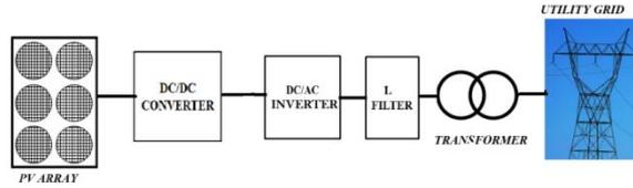
Fig 1. Components of a Grid Connected PV System
