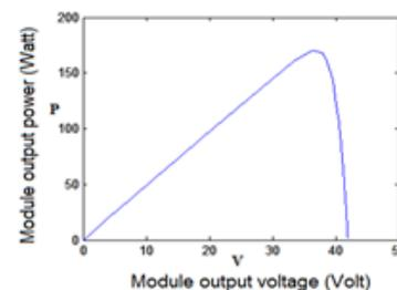
Fig 10. P-V characteristic for PV Module
