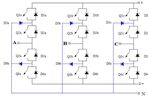
Fig 7. Three phase three level voltage source inverter
