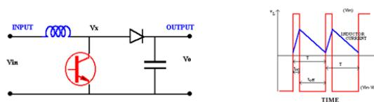
Fig 4. DC-DC boost converter
