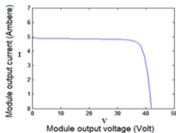
Fig. 9. I-V characteristic for PV Module
