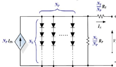
Fig 3. PV module equivalent circuit
