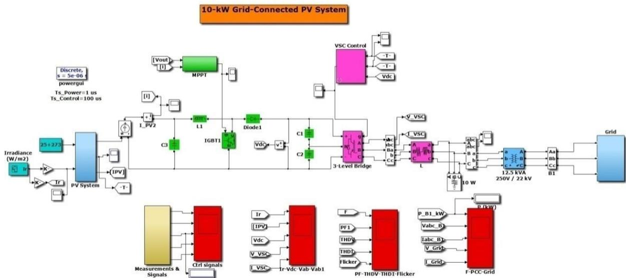
Fig 8. Simulink model for PV system connected to grid
