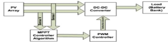
Fig 5. Block diagram of the complete PV structure with MPPT algorithm
