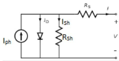
Fig 2. solar cell equivalent circuit
