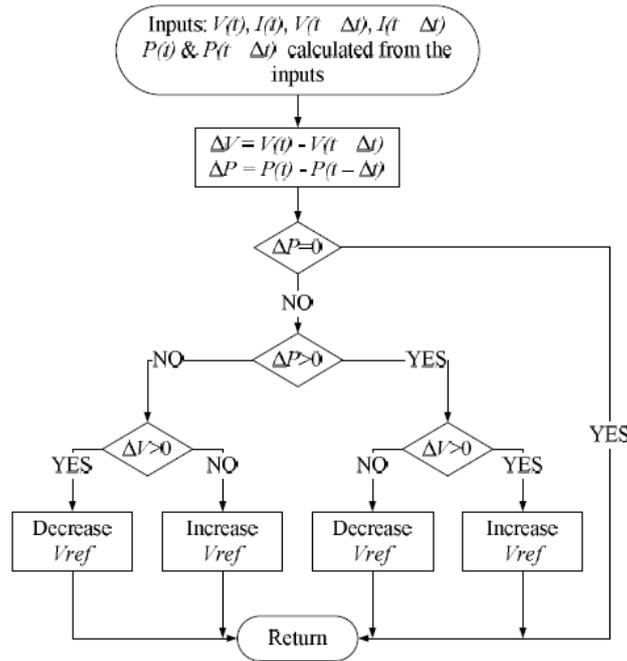
Fig.6 Flow chart for P& O MPPT algorithm
