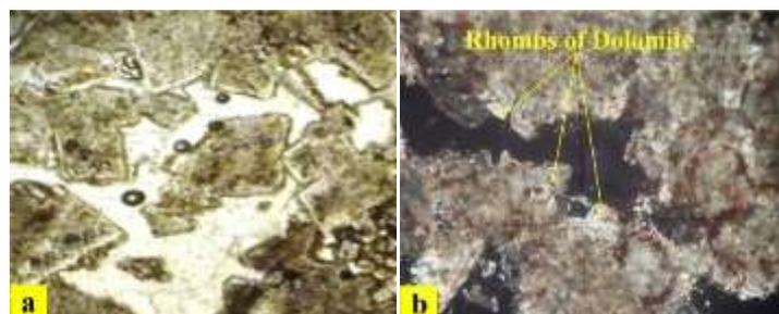
**Figure 10: Photomicrograph of dolomitization process, a: Dolomite site 2M (sample no.2M-
