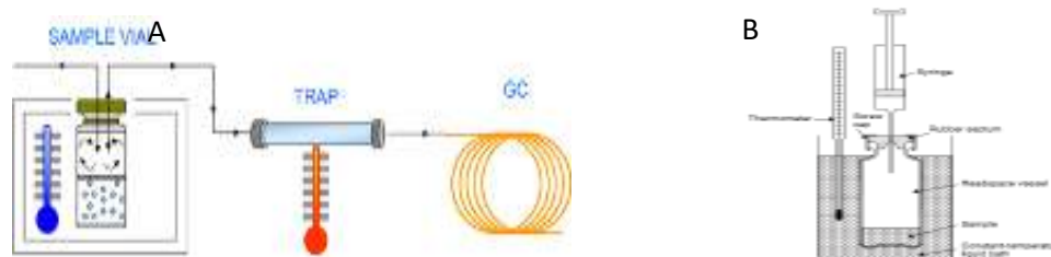
Figure (1), (A) Dynamic headspace & (B) Static headspace sampling (Drawing from Chromservis s.r.o & Hachenberg & Schmidt 1977)
